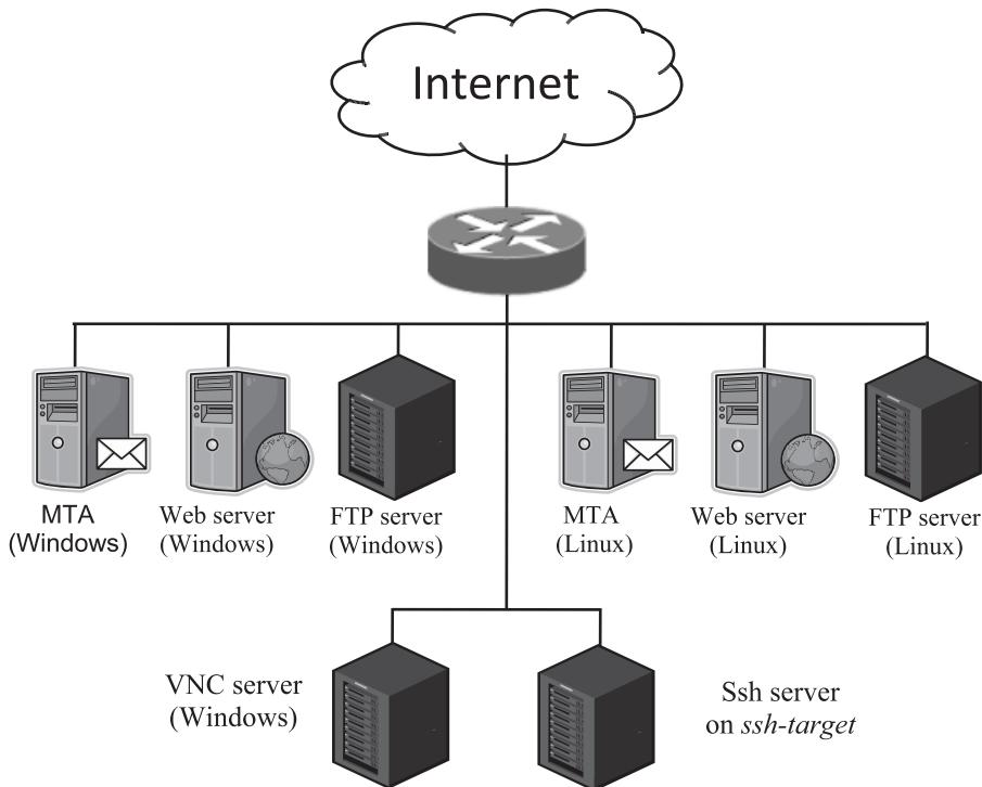
Figure 2. Virtual infrastructure made visible by the honeypot system.
