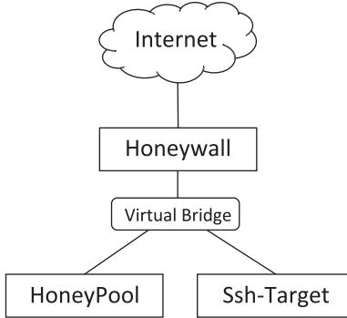
Figure 1. Honeypot system: Virtual machines of the honeypot setup and their interconnection.
