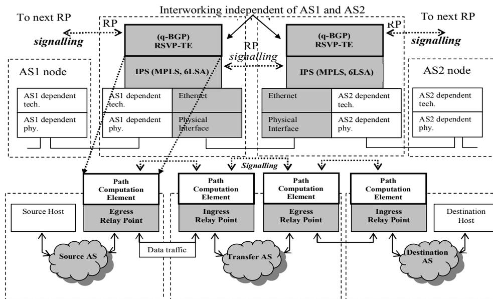
Fig. 2 IPS-centric Relay Point: protocol stack and control plane (in bold).
