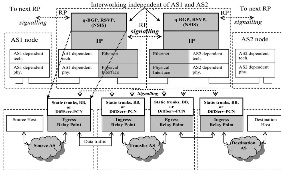
Fig. 1. IP-centric Relay Point: protocol stack and control plane (in bold).
