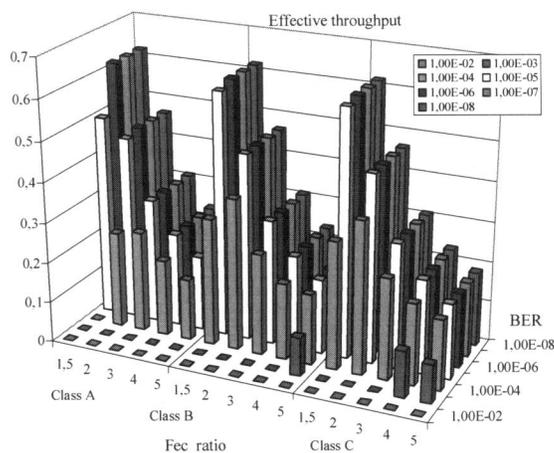
Fig. 5. Effective Throughput measured for different classes of traffic
