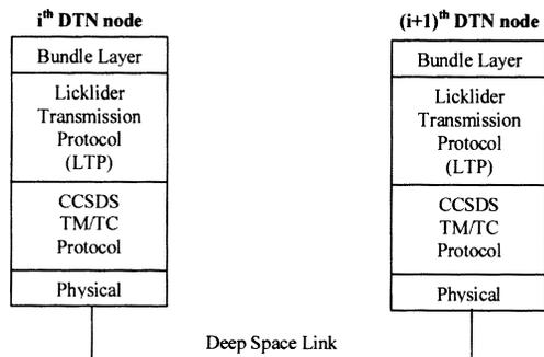
Fig. 1. The Delay Tolerant Network Architecture between two consecutive DTN nodes
