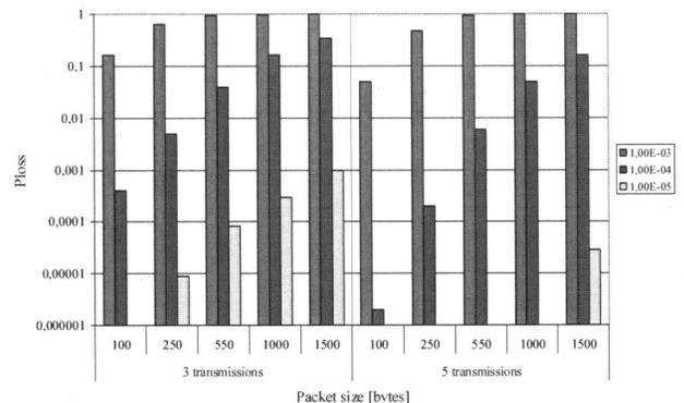
Fig. 3.  $P_{\text{loss}}$  obtained when 3 and 5 transmissions are performed
