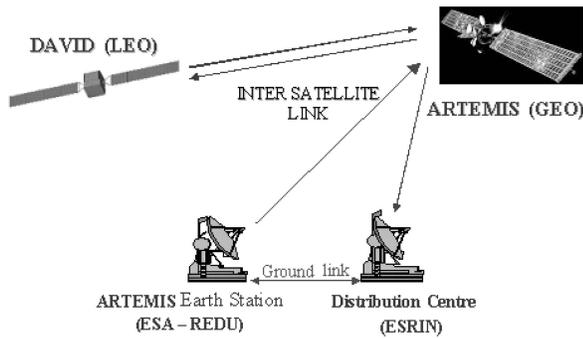
Fig. 10. LEO to end terminal path.
