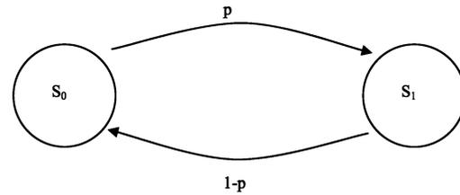
Fig. 11. Two-state channel model.
