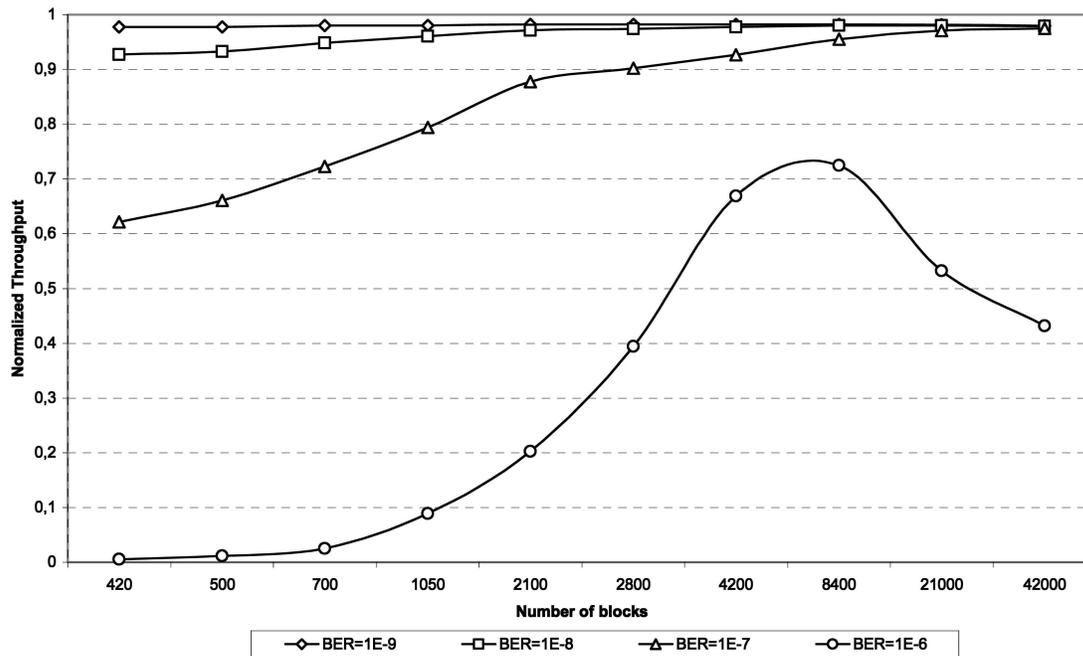
Fig. 8. CFDP reliable NAK immediate normalized throughput.
