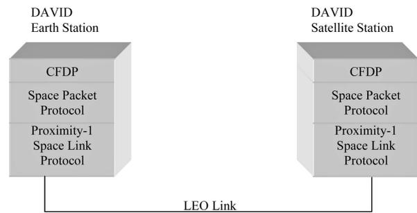
Fig. 7. CFDP-based solution architecture.
