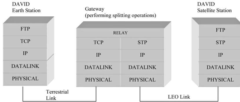
Fig. 5. Splitting architecture.
