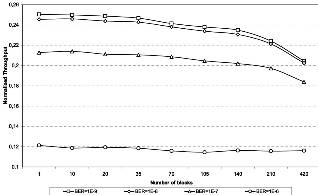
Fig. 3. TCP-IW2-64K normalized throughput.
