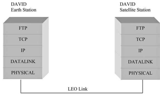
Fig. 2. TCP-based protocol stack architecture.
