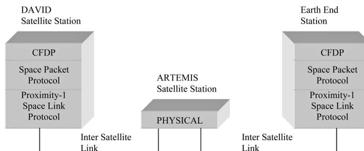
Fig. 12. CCSDS-based protocol architecture.
