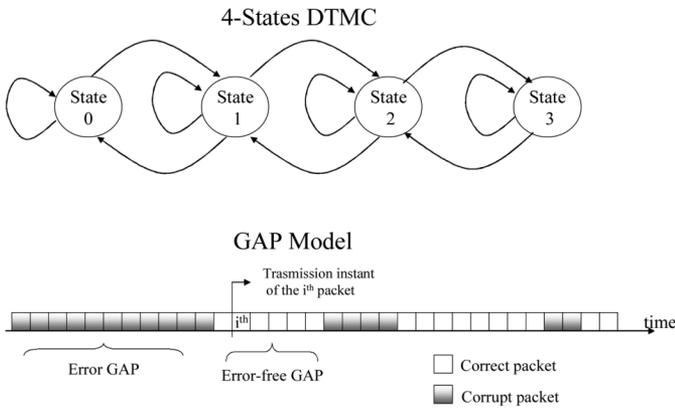
Fig. 2. Four-states/GAP channel model.
