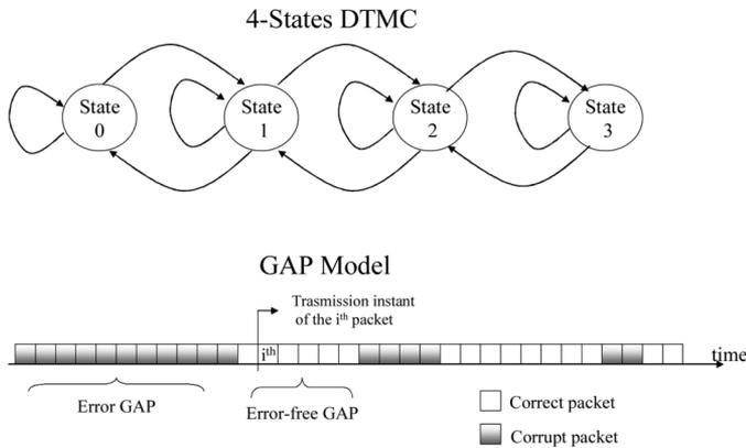
Fig. 2. Four-states/GAP channel model.
