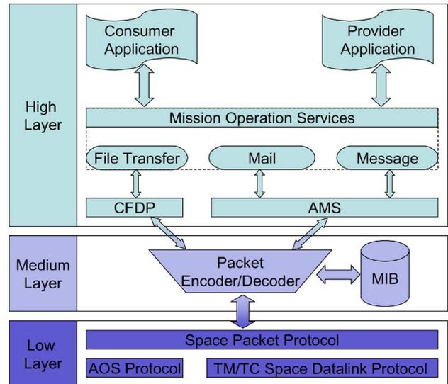
Fig. 3. Reference protocol architecture.
