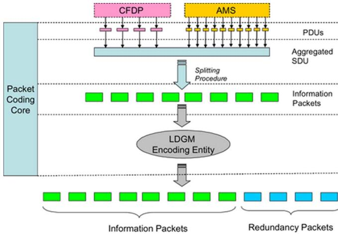
Fig. 4. Packet coding core.
