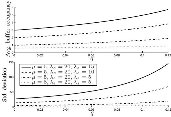
Fig. 3. Average buffer occupancy and its standard deviation for the class of forwarding strategies (12), by varying the parameter  $q$  and considering a model for the endogenous component  $\{g_{k,s}\}$  for which one has  $G'_s(1) = -1$  and  $G''_s(1) = 2$ .
