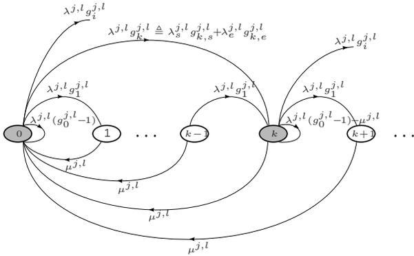
Fig. 2. Transition rates for the continuous-time Markov chain related to  $l$ -queue inside node  $j$ .
