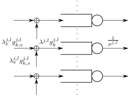
Fig. 1. Model of the generic ICN node  $j \in \{1, \dots, M\}$  and its  $l$ -queue, where  $l \in \mathcal{L}(j)$  ( $k \in \mathbb{N}_0$ ).
