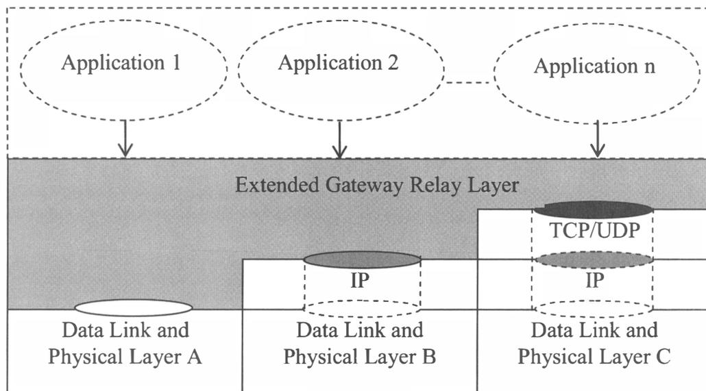
**Fig. 5. Extended Gateway architecture**
