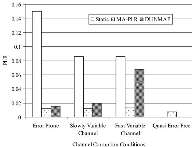
Fig. 3. PLR Comparison in Satellite Channel Corruption Condition.
