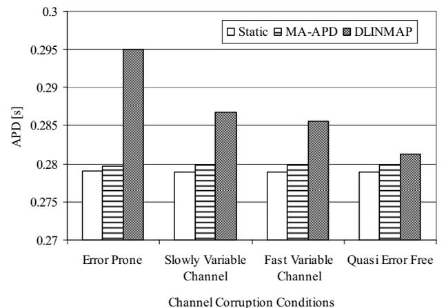
Fig. 2. APD Comparison in Satellite Channel Corruption Condition.
