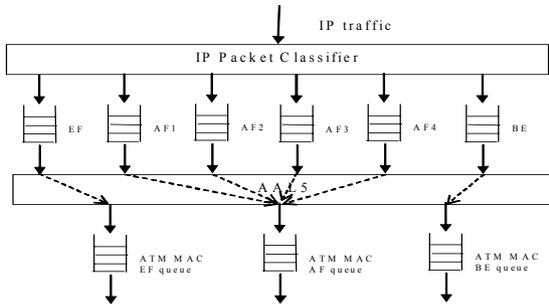
Figure 2. SI-SAP interface. SI layer (DiffServ) over SD layer (ATM). [3, 5].
