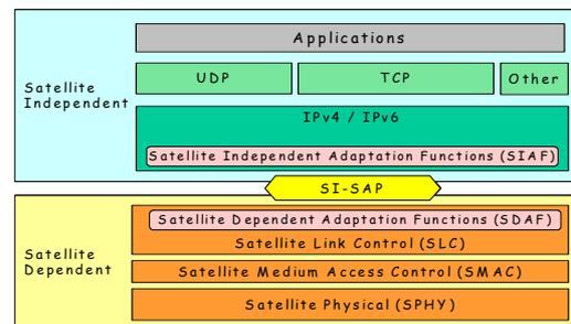
Figure 1. ETSI BSM Protocol Architecture. [1, 2].
