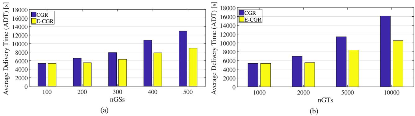
Fig. 2: ADT obtained by using CGR and E-CGR changing  $nGSs$  (a) and  $nGTs$  (b)
