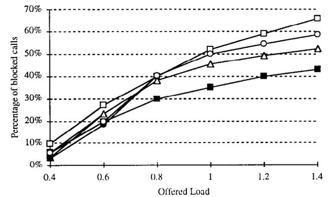
Fig. 14. Overall percentage of blocked calls versus offered load, classes 2 and 4 (for key see Fig. 10).
