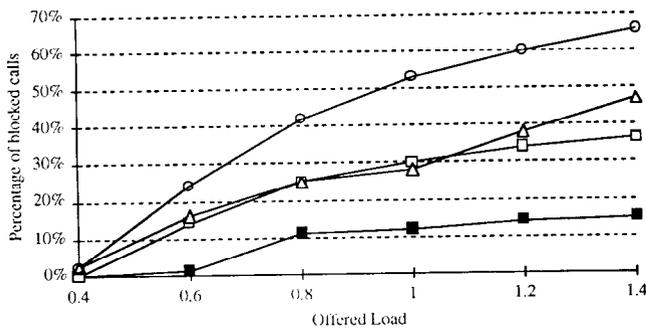
Fig. 11. Overall percentage of blocked calls versus offered load, classes 3 and 4 (for key see Fig. 9).
