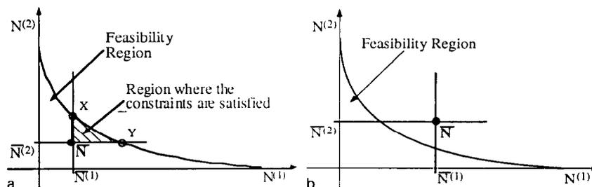
Fig. 4. Effect of constraints (10) on the feasibility region in the case of (a)  $\bar{N} \in F_R$ ; and (b)  $\bar{N} \notin F_R$ .
