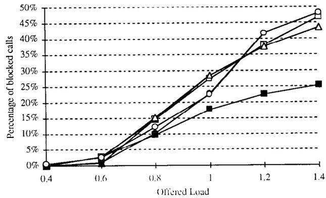
Fig. 10. Overall percentage of blocked cells versus offered load, classes 1 and 2. ■: ES; □: BES; ▲: CSR,  $a = 0.2$ ; △: RSR,  $a = 0.2$ ; ●: CSR,  $a = 0.4$ ; ○: RSR,  $a = 0.4$ .
