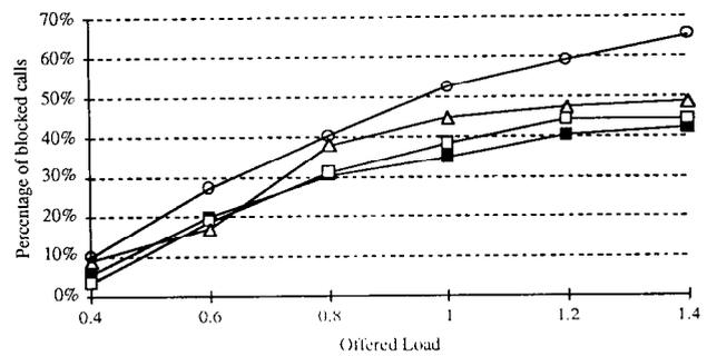
Fig. 13. Overall percentage of blocked calls versus offered load, classes 2 and 4 (for key see Fig. 9).
