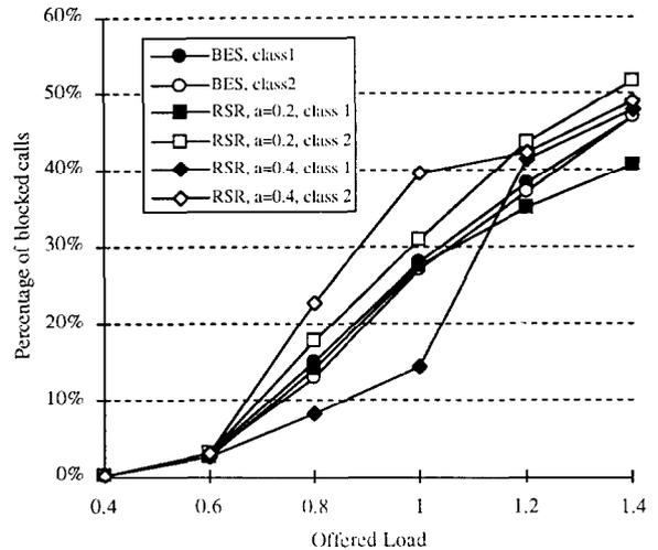
Fig. 16. Percentage of blocked calls for each traffic class vs. offered load, using the BES, RSR with  $a = 0.2$  and RSR with  $a = 0.4$ , for couple A.
