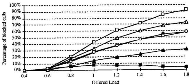
Fig. 15. Percentage of blocked calls for each traffic class vs. offered load, using the ES, FRS and BES for couple A. ■: ES Class 1; □: ES Class 2; ▲: FRS Class 1; △: FRS Class 2; ●: BES Class 1; ○: BES Class 2.
