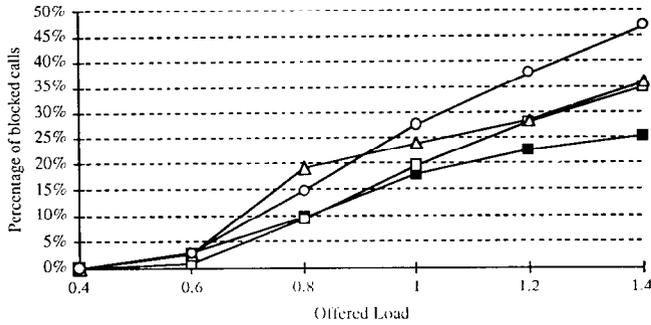
Fig. 9. Overall percentage of blocked cells versus offered load, classes 1 and 2. ■: ES; □: FRS; △: RS; ○: BES.
