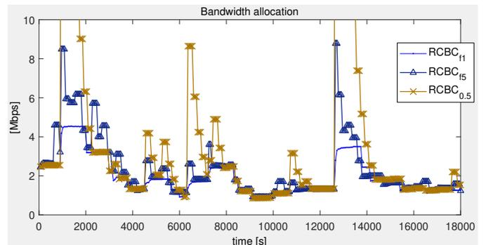
Fig. 2. RCBC bandwidth allocation over time.
