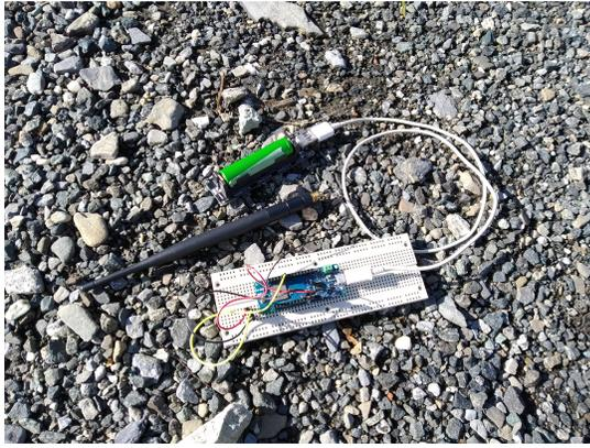
Figure 4: IoT devices based on Arduino MKR WAN 1300
