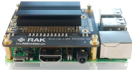
Figure 5: IoT gateway based on Raspberry Pi and RAK 2245 Pi-Hat
