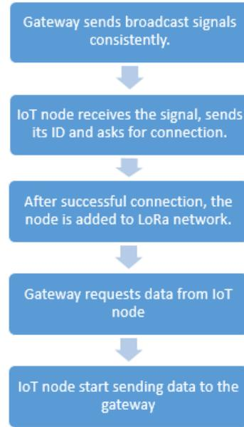
Figure 7: Communication between IoT node and gateway
