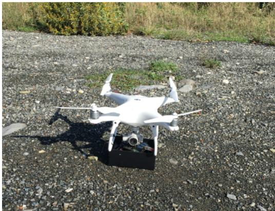
Figure 6: UAV equipped with the IoT gateway
