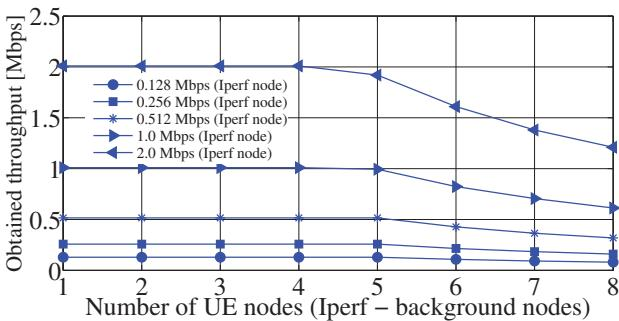
Fig. 4. Obtained throughput for different transmitting data rates of the *Iperf* node vs different number of background nodes.
