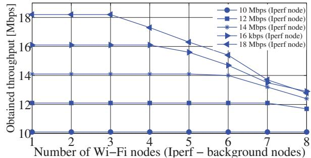
Fig. 6. Obtained throughput for different transmitting data rates of the *Iperf* node vs different number of background nodes.
