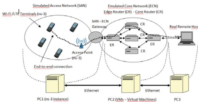
Fig. 2. Hybrid Simulated-Emulated Platform (HySEP) implementation.
