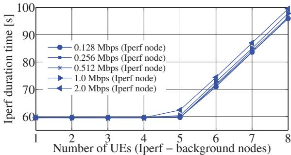
Fig. 3. Iperf transmission time for different transmitting data rates of the *Iperf* node vs different number of background nodes.
