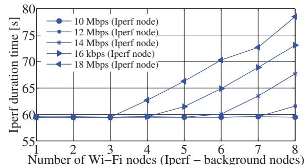
Fig. 5. Iperf transmission time for different transmitting data rates of the *Iperf* node vs different number of background nodes.
