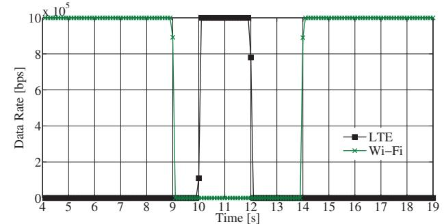
Fig. 9. Received data rate measured by the remote host for Scenario 2 (S2).
